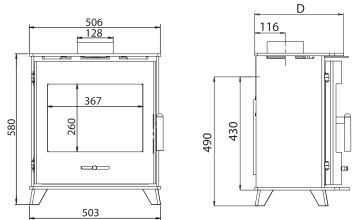
40FS D = 338mm 50FS D = 377mm 60FS D = 434mm All Measurements in mm
