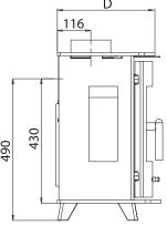
40FS D = 338mm 50FS D = 377mm 60FS D = 434mm All Measurements in mm
